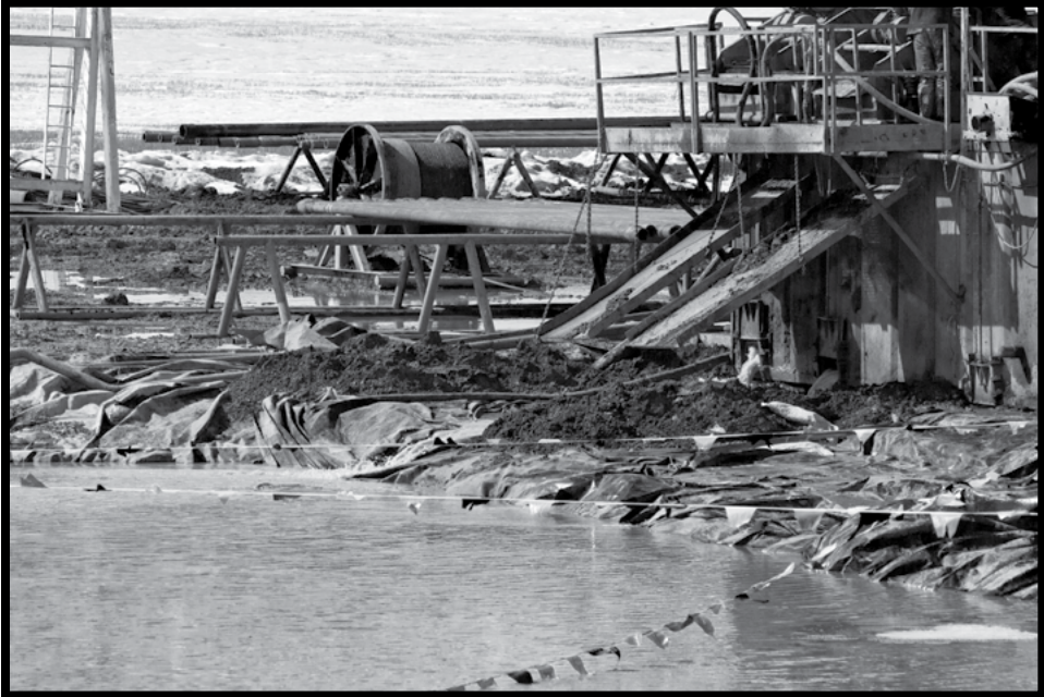
TOXIC This “mud pit” is filled with a slurry of water and diesel fuel, used in the drilling process. Flags are strung across the pond to discourage waterfowl from landing on the toxic liquid. WELLS Contaminants are thought to enter the Poplar River miles upstream, eventually ending up in the city of Poplar’s water supply wells.
