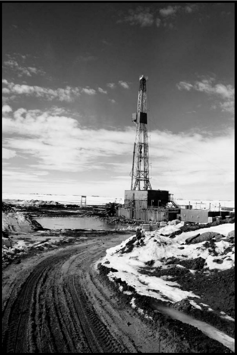
DRILL Drilling rigs like this one operated by DHS Drilling Co. are capable of drilling up to 25,000 feet into the earth. Most wells drilled in the Poplar oil field are around 10,000 feet deep.
